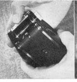
Remove the entire back of the camera by sliding the lock in the direction indicated by the arrow.
