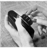
On the top of the lens mount are three markings: BRIGHT (f:16), CLOUDY (f:11), COLOR (f:9.7). Slide the movable pointer opposite the one which applies (see exposure guide).
