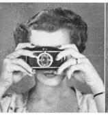
For horizontal pictures, hold the camera as shown above . . . sight through the view-finder, and press the exposure lever smoothly. BE SURE TO HOLD CAMERA STEADY.
