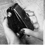
Replace the back, making sure the lock is secure to avoid accidental fogging of the film.
