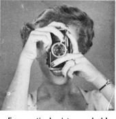
For vertical pictures, hold the camera as shown above . . . sight through the view-finder, and press the exposure lever smoothly. BE SURE TO HOLD CAMERA STEADY.
